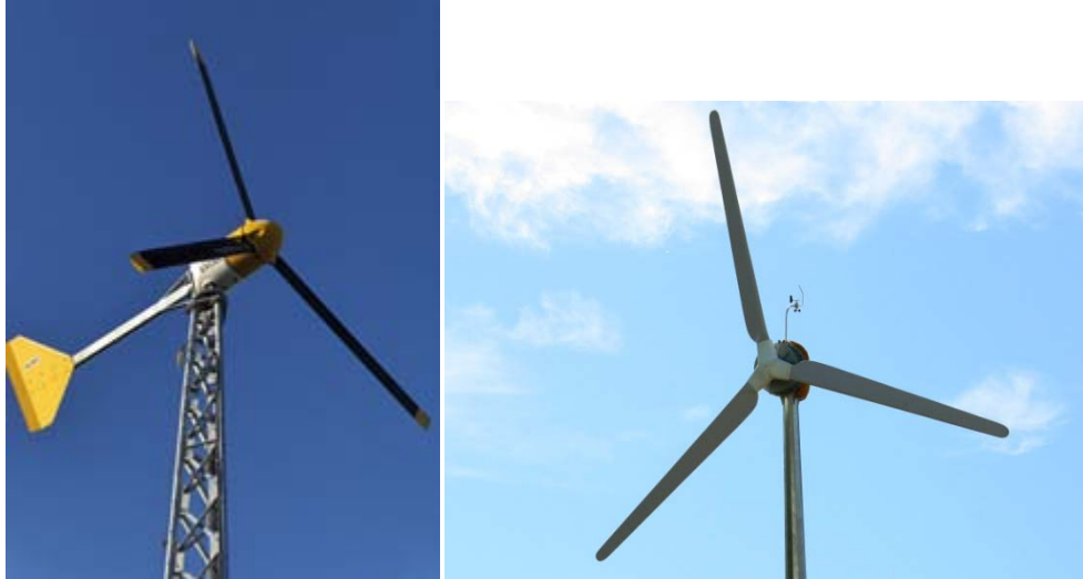
Figure 3 Horizontal Axis Turbines (Bergey 10kW and ReDriven 20 kW)
