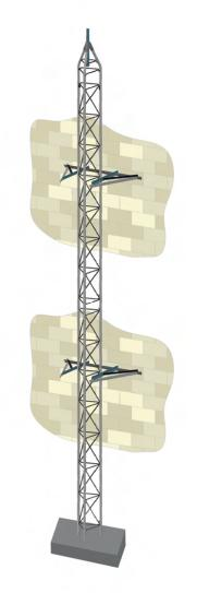
Typical installation on short base with (2) HBUTVRO brackets. (Refer to G-Series accessories for short base)
