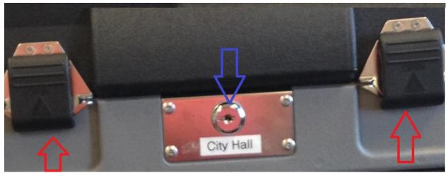
**4.** Unlock the screen to the DS-200 and lift it up gently on the black lid until at 90 degrees.
