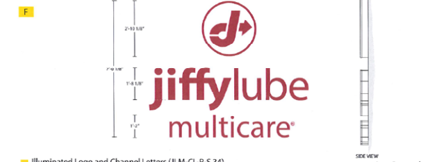
Illuminated Logo and Channel Letters (JLM-CL-R-S-34) Square Feet: 57.68 sq. ft. Scale: 1/2" = 1'-0" 5" deep aluminum channel letter with polished white returns and 1" white jiffylube interscap. "Logo" face to be clear modified acrylic. Logo has 3M 3600-2395 Dark Red vinyl applied first surface overlaid w/ 3M 180MC-10 (30% white vinyl). 70% white diffuser applied second surface. "Letters" face to be clear modified acrylic. Logo has 3M 3600-2395 Dark Red vinyl applied first surface 70% white diffuser applied second surface. Registration Mark is aluminum plate painted MP 43202 White w/ 3M 1622-180 Dark Red opaque vinyl illuminated with Principal White LEDs.
