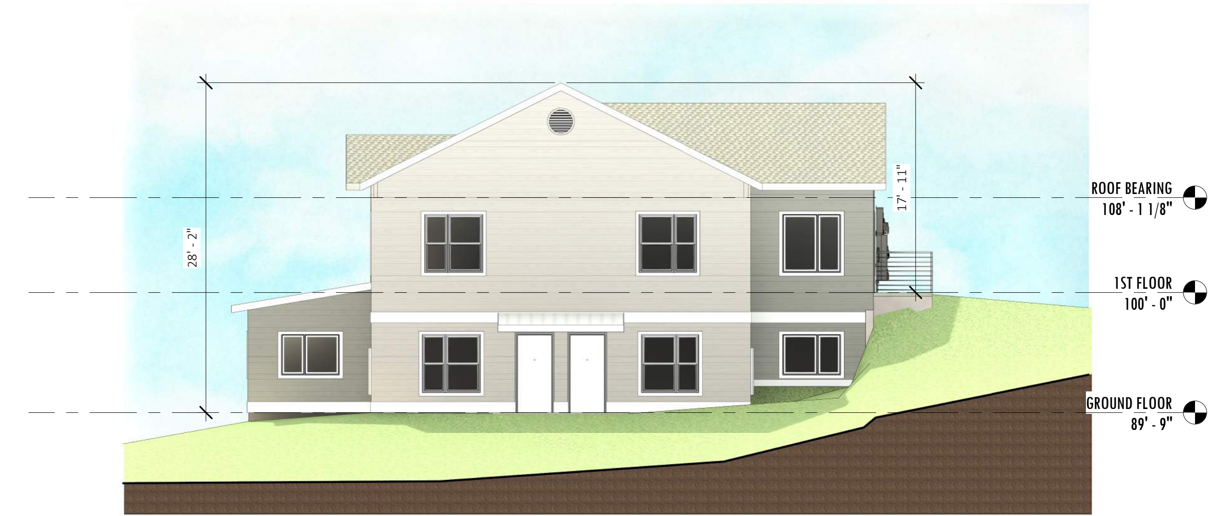
3 BUILDINGS 1, 3, 5, 7 - EAST ELEVATION A2.1 SCALE: 1/8" = 1'-0"
