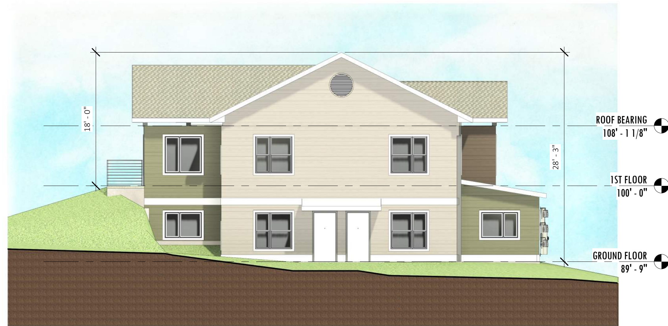
4 BUILDINGS 4 & 6 - WEST ELEVATION SCALE: 1/8" = 1'-0"
