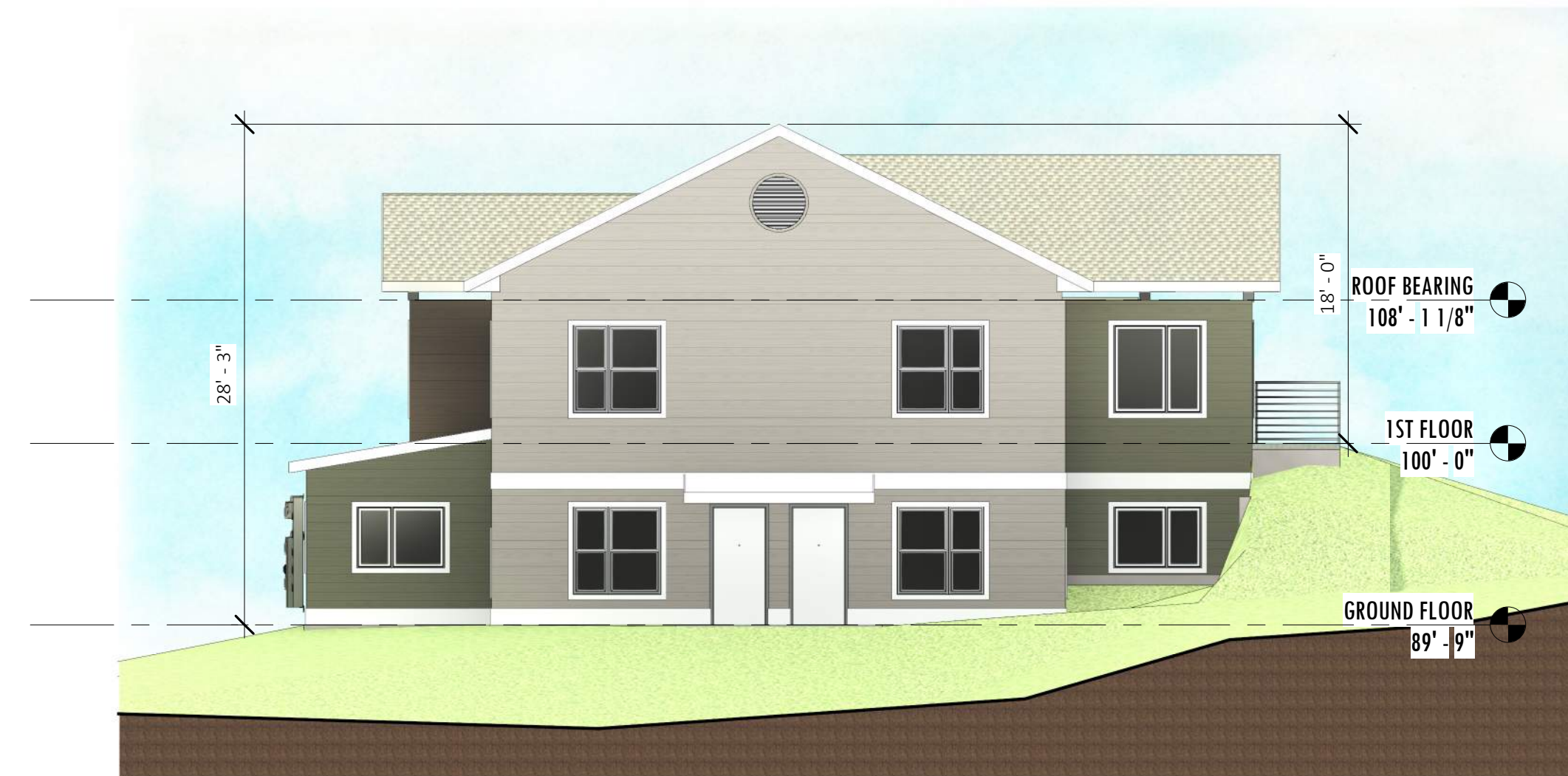
3 BUILDINGS 4 & 6 - EAST ELEVATION SCALE: 1/8" = 1'-0"
