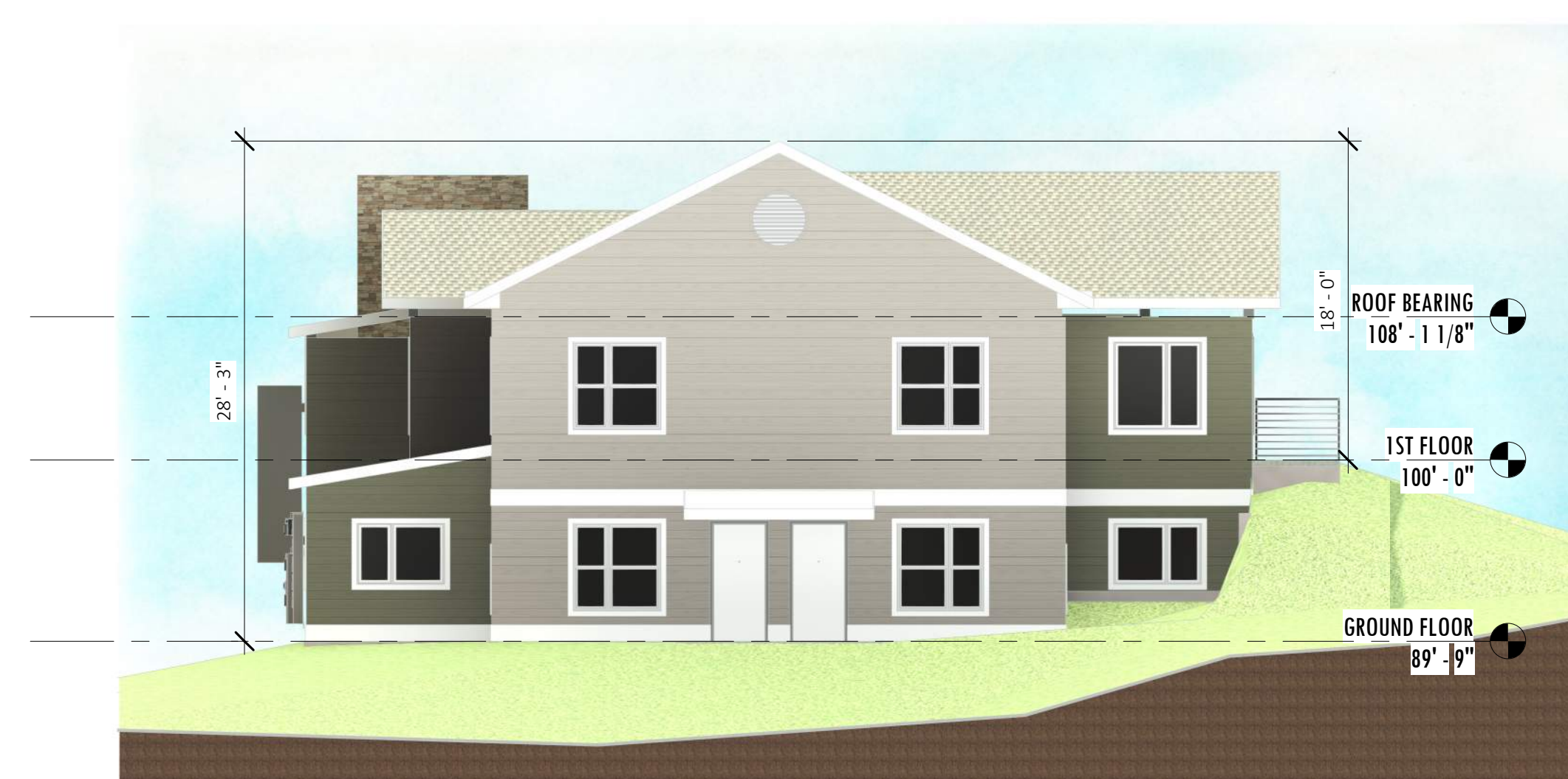
3 A2.2 BUILDING 2 - EAST ELEVATION SCALE: 1/8" = 1'-0"
