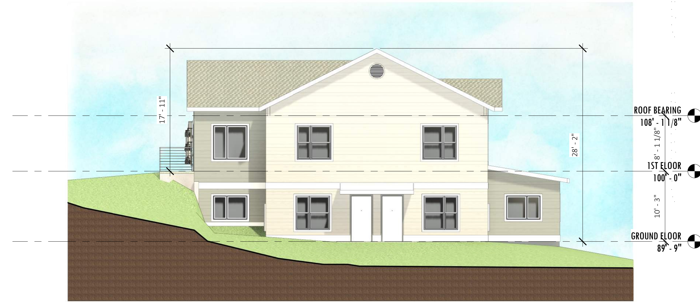
4 BUILDINGS 1, 3, 5, 7 - WEST ELEVATION A2.1 SCALE: 1/8" = 1'-0"
