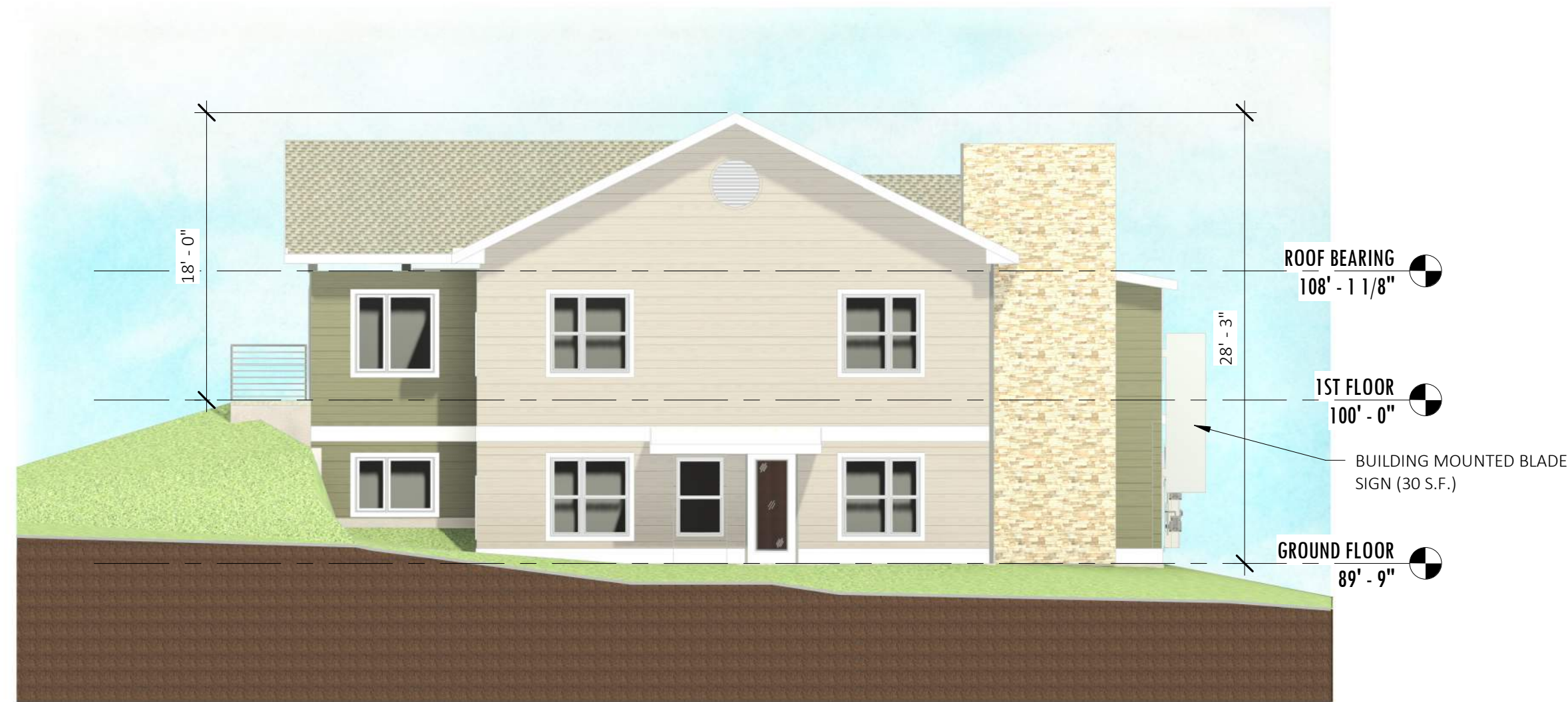
4 A2.2 BUILDING 2 - WEST ELEVATION SCALE: 1/8" = 1'-0"
