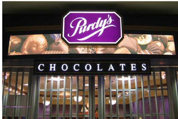
When a script font is used, the size of the lettering - and, thus, the size of the sign itself - must be increased to ensure readability.
