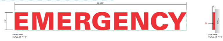
CL.2 36" FACE LIT CHANNEL LETTERS - REMOTE POWER SUPPLY - EXTERIOR (QTY 1) SQUARE FOOTAGE: 87.9
